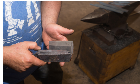
Each blade starts as a rough stack of steel plates that are repeatedly heated, stretched folded and cut to create hundreds of layers of steel in each blade.
